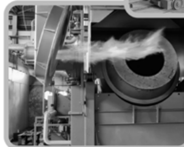
TRF : Tilting Rotary Furnace
